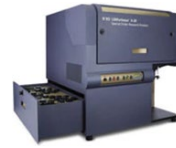
Flow cytometry analyzer up 30 parameters / 5 lasers (BD Canto II, BD Fortessa X20, Biorad ZE5 and BD Symphony)
