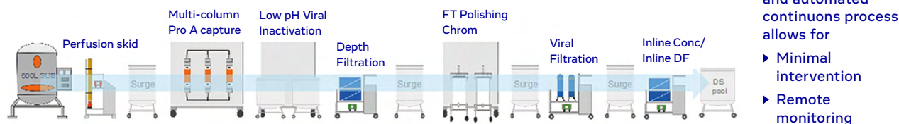
Figure 6: Traditional fed-batch process (top) compared to Just – Evotec Biologics continuous process for mAb production (bottom).
