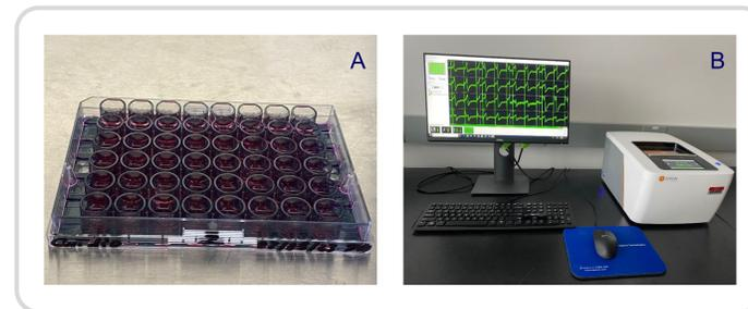
Figure 1: A. Biocircute 48-well/16 electrodes plate. B. AXION MAESTRO PRO research platform.
